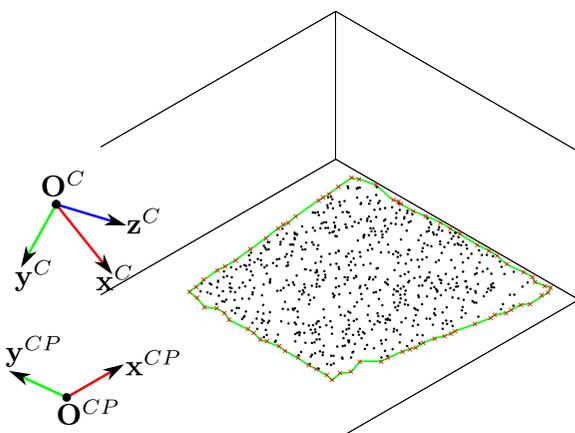
**Fig. 5** Example the  $\alpha$ -shape output result with red Xs being the edges, black points the point set and green lines the polygon
