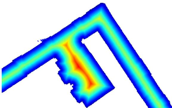
**Fig. 9** Example of a distance-to-obstacles grid map
