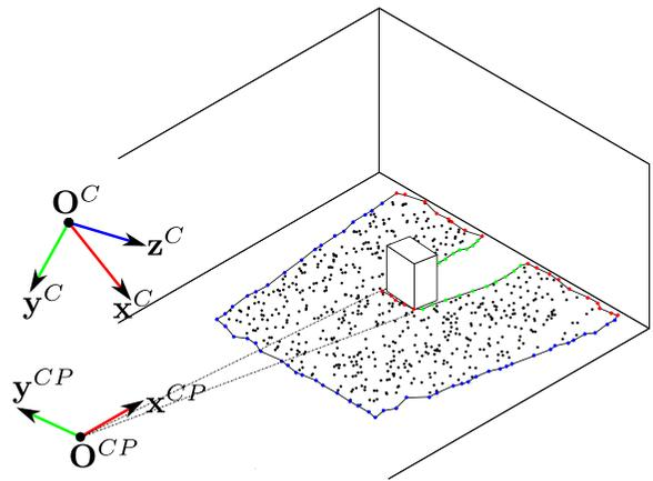
**Fig. 6** Example of the edges resulted from the  $\alpha$ -shape algorithm differentiating the type of edges: in red/grey the environment edges, in blue/black the FOV limits edges and in green/dashed the shadows edges
