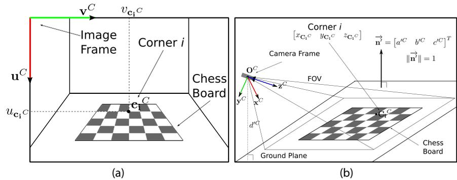
chess pattern is placed in the line of sight of the depth camera, maintaining the robot still. A chess pattern detection algorithm [22] is used to detect the corners pixels on the image. Then we obtain the corresponding 3D points from the point-cloud, that we know are part of the ground-plane.
