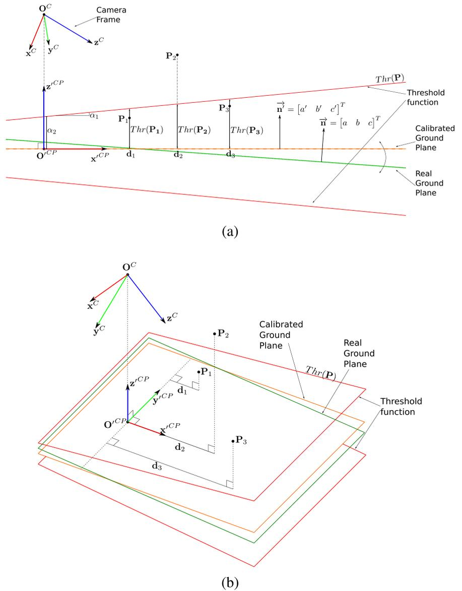
To filter these outliers and to estimate the real ground model parameters,  $(a^C, b^C, c^C, d^C)$ , a RANSAC algorithm is used with the model characterized in (1). The result incorporates the ground point-cloud (points considered as inliers). Figure 1d shows the resulting point-cloud after the dynamic threshold filter and the resulting point-cloud inliers after the RANSAC algorithm.
