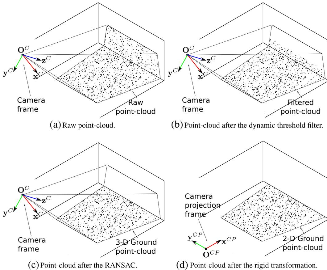
**Fig. 1** Illustration of the ground point-cloud detection algorithm steps
