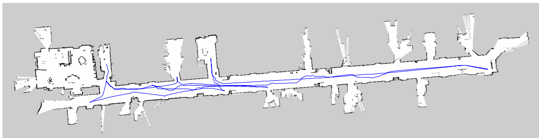
Fig. 7. Trajectory of ISR-CoBot autonomously navigating along the IPOL premises. The task consisted in a sequence of waypoints.
